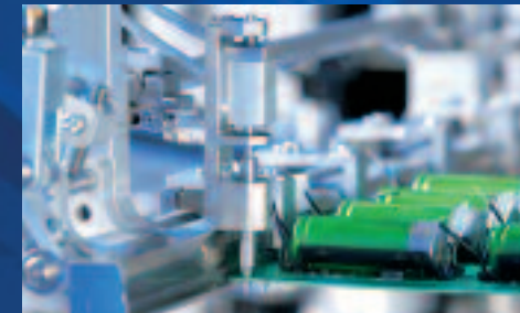
Location pin for positioning PCB
